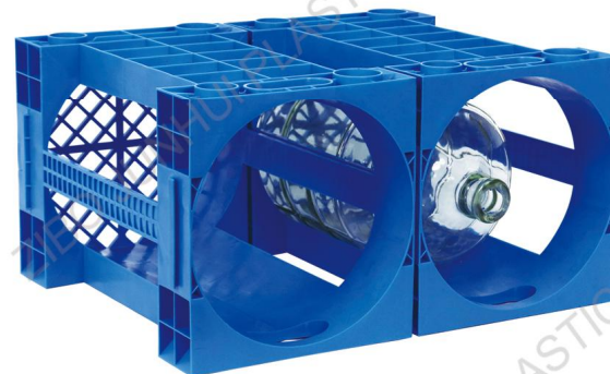
387-292 plastic crate External size: 387*387*292mm Internal size: 356*356*278mm Weight: 1.72kg
